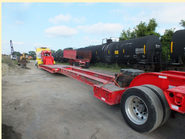
Special Low Boy trailer that expanded from 40 feet long to 90 feet long.
