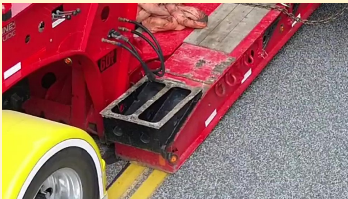
Lowered the Low Boy and lowered the air cushion ride
